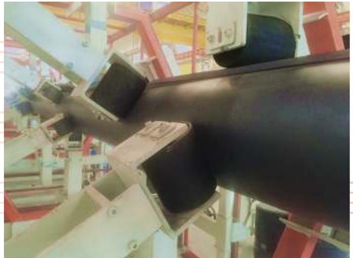
MAXX STEELFLEX™ MAXX ROUND<sup>®</sup> - Pipe Belts with steel cord reinforcement
