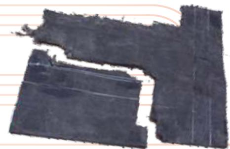
Longitudinal rip arrested by **MAXX SHIELD**®
